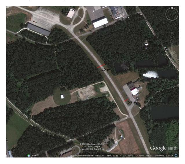
The obstacle wingtip clearance (according to ICAO Annex 14) on taxiway "E" is only assured for aircraft with a wingspan of  $\leq$  15 m.
